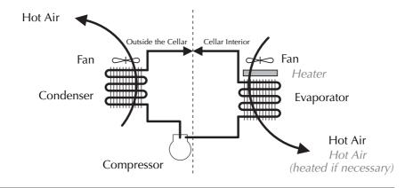
The EuroCave CL-A/B air conditioner is a cooling unit with a fan that causes the air to flow around the bottles in your cellar. The air is then sucked up into the evaporator where it cools down again and loses part of the moisture it contains before starting a new cycle.
