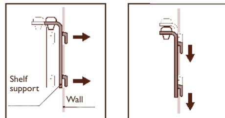
To change the position of a sliding shelf, first completely unload the shelf. Then lift the sliding shelf and slide it towards you whilst holding the front of it upwards. Remove the wall slider guides, marking which is right and which is left, then reinstall them as shown below:
