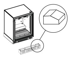
When the cabinet is installed with the hexagonal raising pieces to be elevated, you must adapt the shape of the separators. This is important in order to correctly guide the air flows downwards and therefore to the ventilation grid (incoming or outgoing). The diagram above shows an exemple of shape for the separators, it is not provided with the unit.
