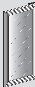
Technical glass door (thickness of the decor panel = 20mm max. weight of the decor panel: 12Kg)
